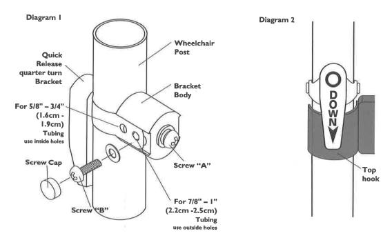
The back is properly secured when the bottom pins are resting in the lower post brackets and the upper NOTE: quick release quarter turn brackets are installed above the back support's top hook brackets with the quick release mechanism pointing down.
