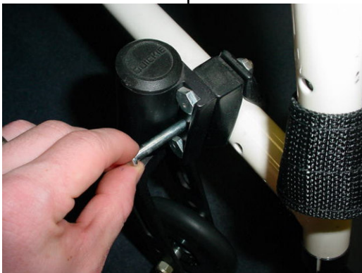
Figure 13: Clevis Pin Location
