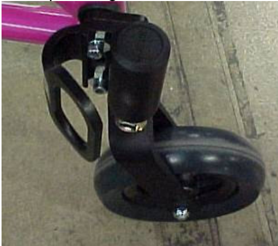
Figure 12: Final Setup with Caster Barrel Leading
