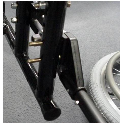
Figure 2: Bolts inserted into Anti Tip And frame.
