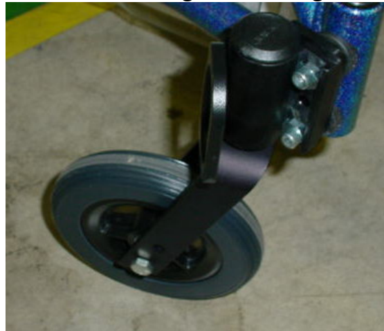
Figure 13: Final Setup with Caster Barrel Trailing
